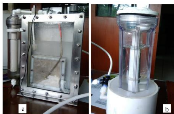
FIGURE 3. Experimental setup for HHO production and gas flow measurement: (a) Overall generator, (b) Flow measurement apparatus.
